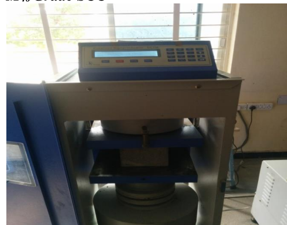
Fig: 7.2 Compressive Testing of SCC Cube Using Digital Compression Testing Machine
