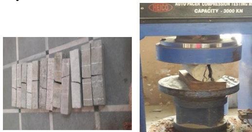
Fig .Tested Beams
