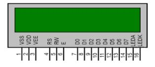
It is called Liquid Crystal Display. We are going to use 16x2 characters LCD. This will be connected to microcontroller. The job of LCD will be to display all the system generated messages coming from the controller. LCD will provide interactive user interface. This unit requires +5VDC for it proper operation. This module is used for display the present status of the system.
