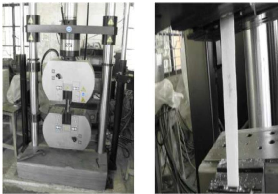
Fig.7 Test of FRP plate in INSTRON 1195
