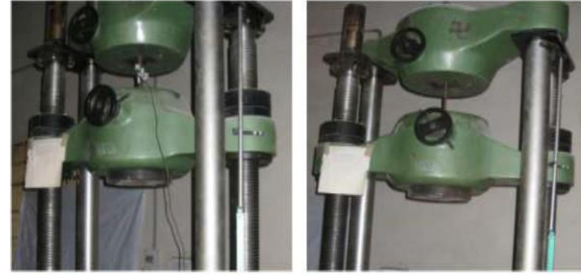
Fig6 Tensile Strength of Steel in Electronic UTM
