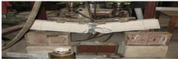
Fig. 5.20 Failure of beam CB1
