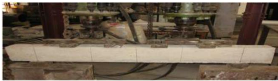
Fig 10 Loading arrangement beam CB1
