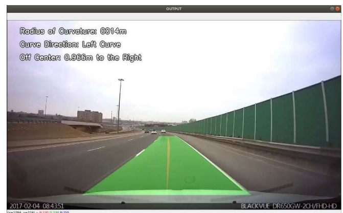
Fig. 7. Lane Detection System Output – Left curve detected
