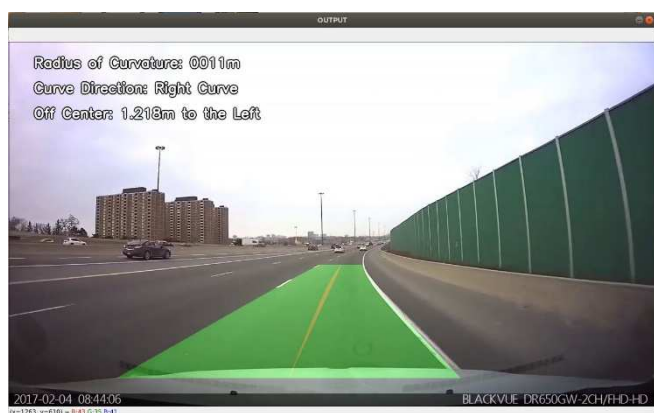
Fig. 9. Right curve detected
