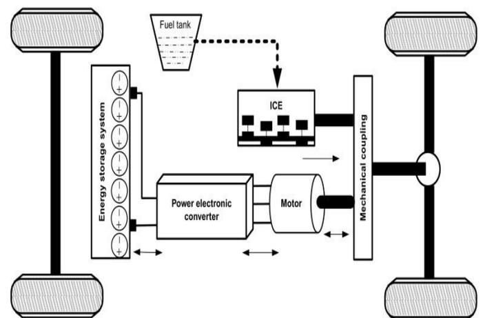
Fig. 1. Schematic diagram of Parallel Hybrid Transmission
