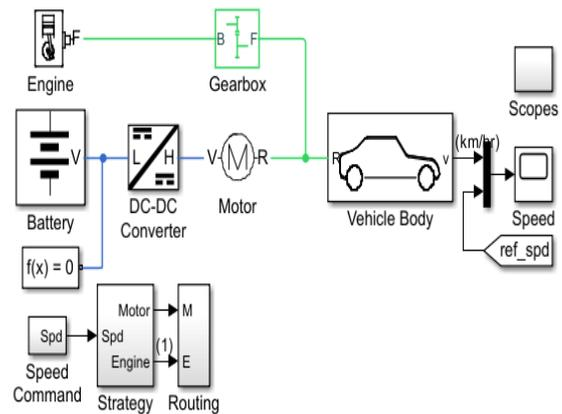
Fig. 3 Basic architecture of a parallel hybrid transmission
