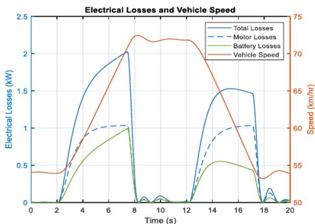
Electrical losses and vehicle speed figure shows that while the vehicle speed is constant, battery and motor losses grow somewhat, and when the vehicle speed is constant and in deceleration mode, battery and motor losses reduce dramatically.
