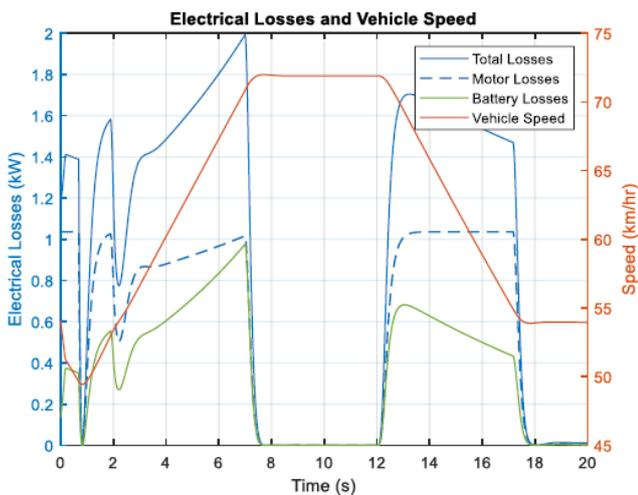
It can be seen from the electrical losses and vehicle speed plot that during the first phase, due to higher power dissipation, motor and battery losses alter as well.
