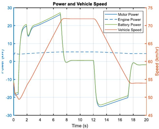
The motor and battery dissipate more power in the initial phase, as shown in the graph above, while the rest of the phases remain the same as before adjusting the follower to base teeth ratio.
