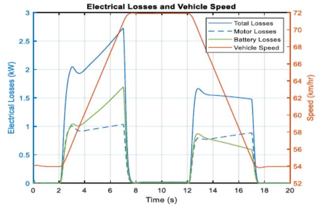
As the DC-to-DC voltage converter's winding ratio grew, the battery voltage decreased. The electrical losses plot shows that battery losses have increased, resulting in an increase in overall electrical losses during the acceleration and deceleration phases. As a result of this experiment, we can deduce that increasing the battery voltage will result in minimal battery losses.
