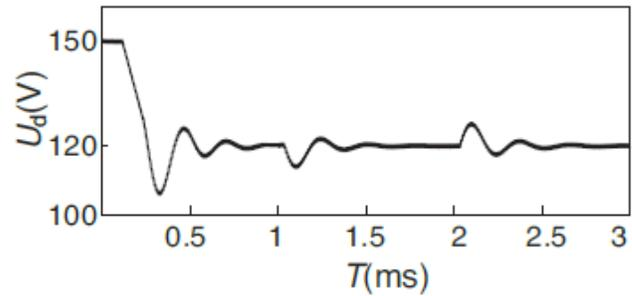
Fig. 10. Waveform of buck mode with load disturbance
