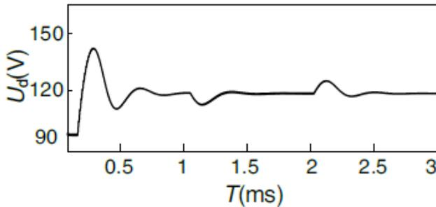
Fig. 9. Waveform of boost mode with load disturbance
