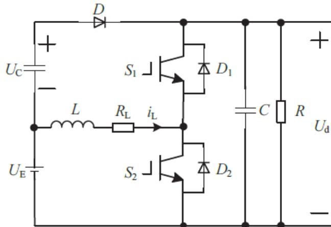
Fig. 4. Equivalent circuit diagram of boost mode
