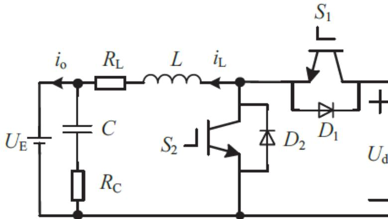
Fig. 3. Equivalent circuit diagram of buck mode
