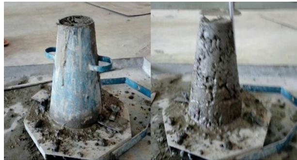
**Figure - 2 Slump test**
