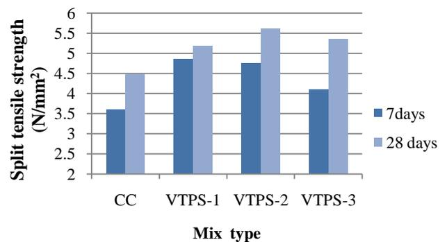
Figure - 7 Split tensile values at 7<sup>th</sup> and 28<sup>th</sup> day
