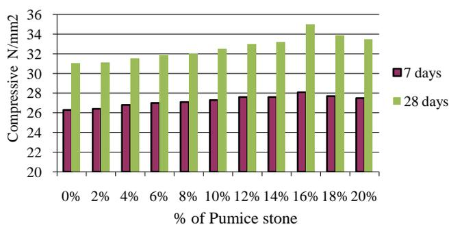
By this sample test high strength obtained at 16% replacement of pumice stone. So followed by the test result
