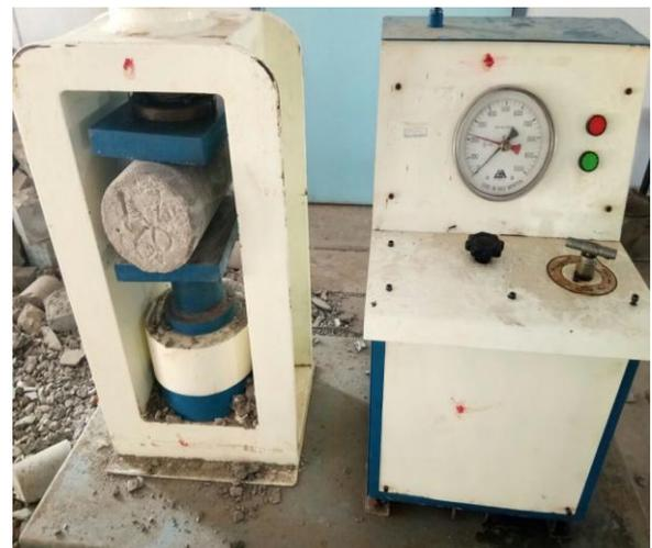
Figure - 6 Split tensile test
