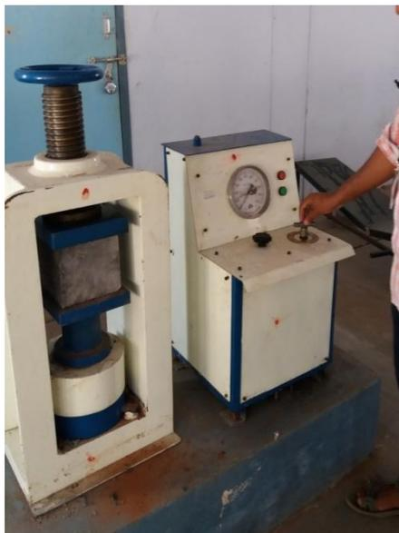
Figure - 4 Compressive strength test
