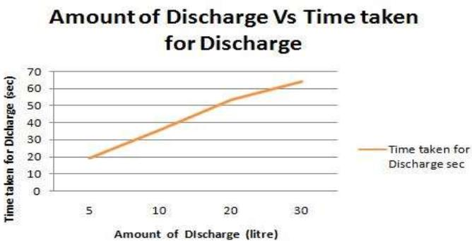
Graph 2. Amount of Discharge Vs Time taken for Discharge
