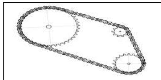
Fig.3. chain drive with additional power output sprocket
