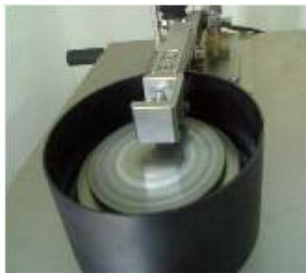
**Fig 3.** Photographic view of pin on disk wear testing machine
